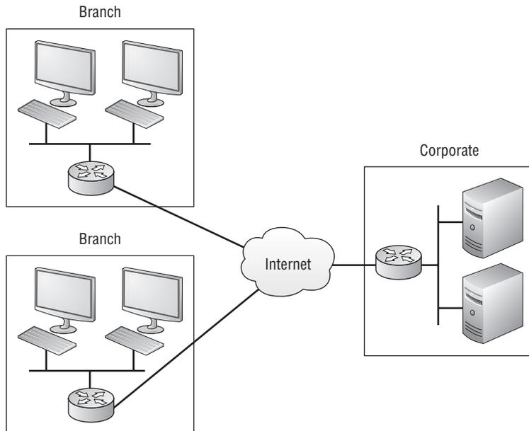
The Internet is a prime example of what's known as a *distributed* WAN—an internetwork that's made up of a lot of interconnected computers located in a lot of different places. There's another kind of WAN, referred to as *centralized*, that's composed of a main, centrally located computer or location that remote computers and devices can connect to. A good example is remote offices that connect to a main corporate office as shown in Figure 1.5.
