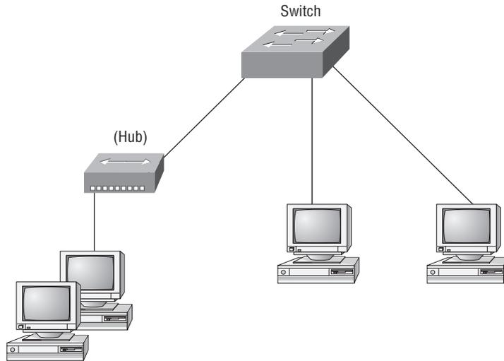
Keep in mind that the hub used in Figure 2.1 just extended the one collision domain from the switch port. Here’s a list of some of the things that commonly cause LAN traffic congestion:
