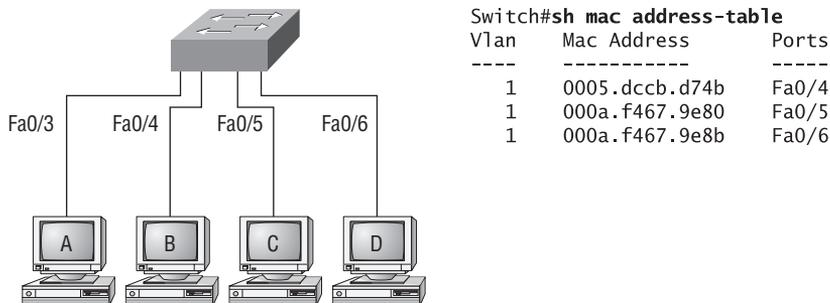
Let's take a look at the output of an IOS-based switch to make sure you've got this foundational concept nailed down before we move to NX-OS. The command on both IOS and NX-OS is `show mac address-table`:
