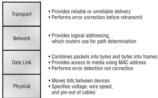
In Figure 2.6, you can see that it's the four bottom layers that define how data is transferred through a physical wire or through switches and routers. These bottom layers also determine how to rebuild a data stream from a transmitting host to a destination host's application.
