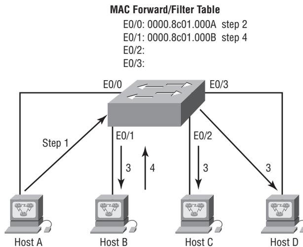
Here, you can see four hosts attached to a switch. When the switch is powered on, there's nothing in its MAC address forward/filter table, but when the hosts start communicating, things begin to change. The switch places the source hardware address of each frame into a table along with the port with which the frame's source address corresponds.
