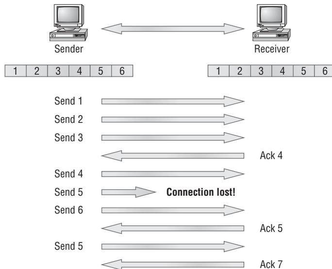
The receiving node acknowledges it has received them by requesting segment 4 with an ACK 4. When it receives the acknowledgment, the sender then transmits segments 4, 5, and 6. If segment 5 doesn't make it to the destination, the receiving node
