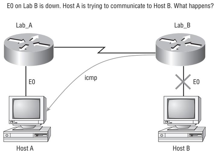
When Host A sends a packet destined for Host B, the Lab\_B router will send an ICMP destination unreachable message back to the sending device (Host A in this example).
