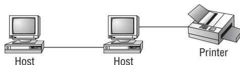
Okay—Figure 1.1 shows a really basic network made up of only two host computers connected together; they share resources like files and even a printer hooked up to one of the hosts. These two hosts “talk” to each other using a computer language called *binary code*, which consists of lots of 1s and 0s in a specific order that describes exactly what they want to “say.”
