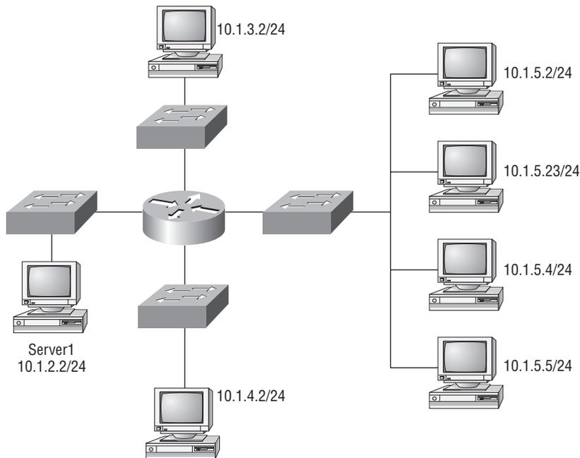
Server1 (10.1.2.24) telnets to 10.1.1.5 from a DOS prompt. What do you think Server1 will receive as a response? Since Server1 will send the Telnet data to the default gateway, which is the router, the router will drop the packet because there isn't a network 10.1.1.0 in the routing table. Because of this, Server1 will receive a destination unreachable back from ICMP.
