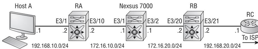
Here you see three Nexus switches, one 7000 series and two 5000 series named RA and RB. RA and RB are preconfigured for this chapter. Also present is RC, which is an ISR router, connecting to an ISP. We're going to focus on configuring the Nexus 7000 in this chapter.
