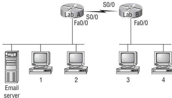
Okay—one more question and you're on your way to being an IP routing genius! Again, using Figure 9.8, Host 4 is transferring a file to the email server connected to the Lab\_A router. What would be the layer 2 destination address leaving Host 4? Yes, I've asked this question more than once. But not this one: What will be the source MAC address when the frame is received at the email server?
