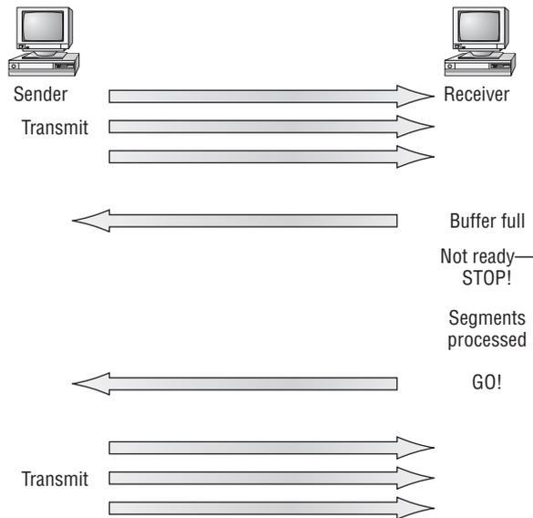
In fundamental, reliable, connection-oriented data transfer, datagrams are delivered to the receiving host in exactly the same sequence they’re transmitted—and the transmission fails if this order is breached! If any data segments are lost, duplicated, or damaged along the way, a failure will occur. This problem is solved by having the receiving host acknowledge that it has received each and every data segment.
