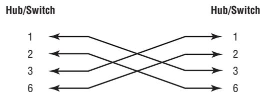
Notice that instead of connecting 1 to 1, 2 to 2, and so on, here we connect pins 1 to 3 and 2 to 6 on each side of the cable.
