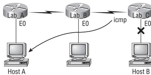
Lab\_C will use ICMP to inform Host A that Host B can't be reached, and it will do this by sending an ICMP destination unreachable message. The point of this figure is to help you visualize how ICMP data is routed via IP back to the originating station.
