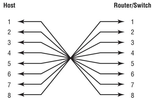
These are probably the easiest cables to make because you just cut the end off on one side of a straight-through cable, turn it over, and put it back on (with a new connector, of course).
