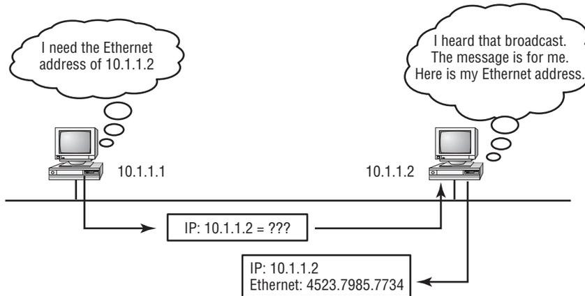
The following trace shows an ARP broadcast—notice that the destination hardware address is unknown and is all *Fs* in hex (all 1s in binary)—and is a hardware address broadcast:
