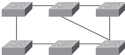
Here you see a switched network with a redundant topology that includes switching loops. Without some type of layer 2 mechanism in place to prevent a network loop, the network could be plagued by any of the problems I just talked about: broadcast storms, multiple frame copies, and MAC table thrashing.
