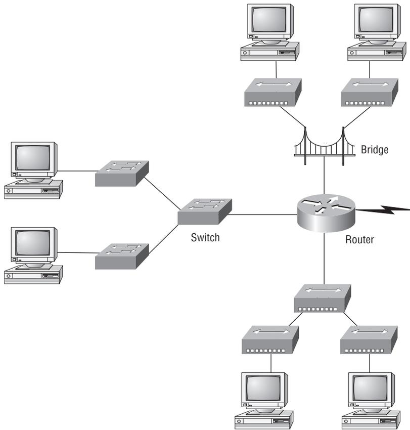
When you looked at Figure 2.3, did you notice that the router is found at center stage and that it connects each physical network together? We have to use this layout because of the older technologies involved—bridges and hubs.
