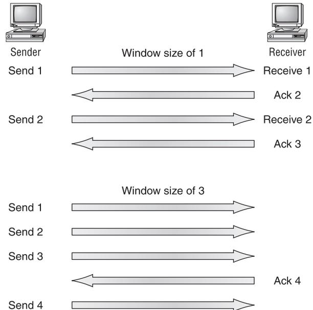
In this simplified example, both the sending and receiving machines are workstations. In reality, this is not done in simple numbers but in the amount of bytes that can be sent.
