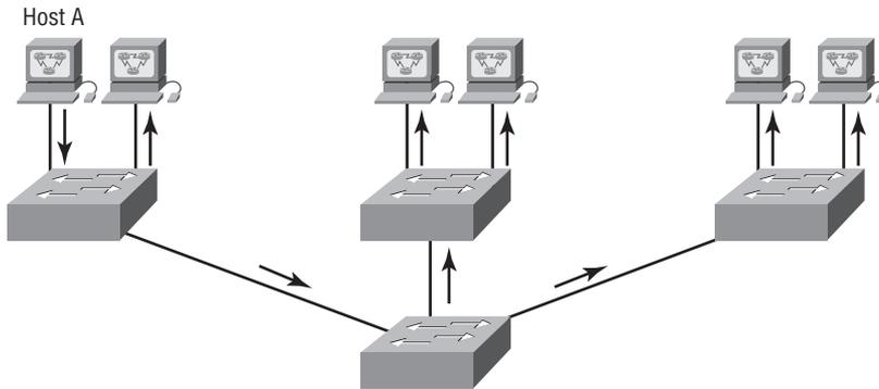
**FIGURE 11.5** The benefit of a switched network
