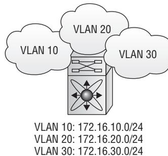
As you know, the hosts in these three VLANs can't communicate to hosts outside their own VLAN by default. I just addressed this issue by connecting a router port into each VLAN and then configuring "router on a stick."
