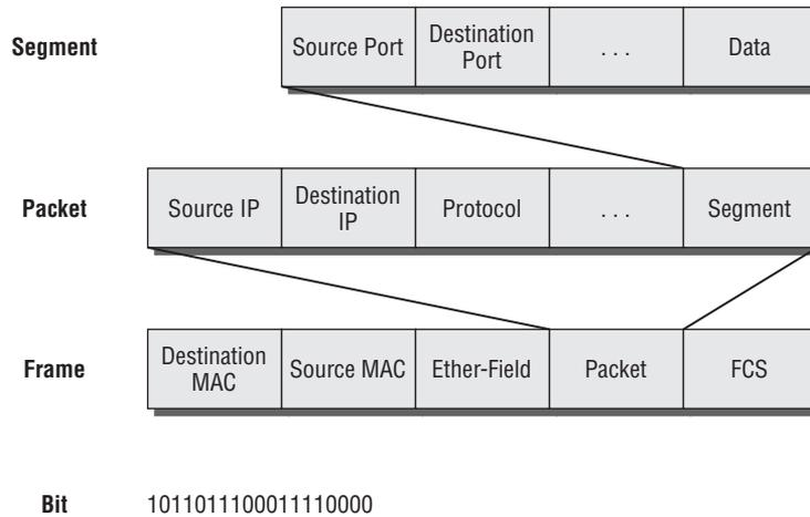
**FIGURE 3.14** Port numbers at the Transport layer
