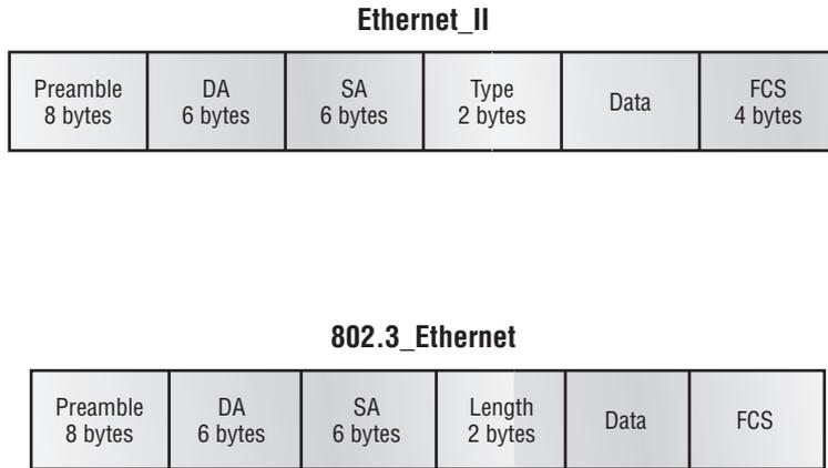
**Destination Address (DA)** This transmits a 48-bit value using the least significant bit (LSB) first. The DA is used by receiving stations to determine whether an incoming packet is addressed to a particular node. The destination address can be an individual address or a broadcast or multi-cast MAC address. Remember that a broadcast is all 1s (or *Fs* in hex) and is sent to all devices but a multicast is sent only to a similar subset of nodes on a network.
