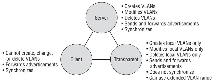
**Server** This is the default mode for all Catalyst switches. You need at least one server in your VTP domain to propagate VLAN information throughout that domain. Also important: the switch must be in server mode to be able to create, add, and delete VLANs in a VTP domain. VLAN information must be changed in server mode, and any change made to VLANs on a switch in server mode will be advertised to the entire VTP domain. In VTP server mode, VLAN configurations are saved in NVRAM on the switch.
