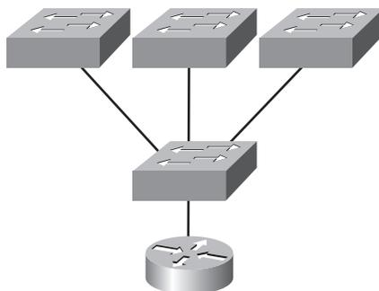
Router connecting all VLANs together allowing for inter-VLAN communication, using only one router interface (router on a stick).
