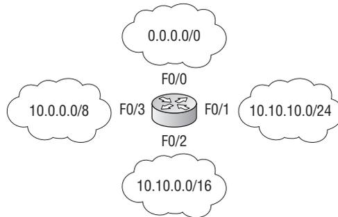
By using the command `show ip route` on an IOS router we can see the routing table (map of the internetwork) that Lab\_A uses to make forwarding decisions:
