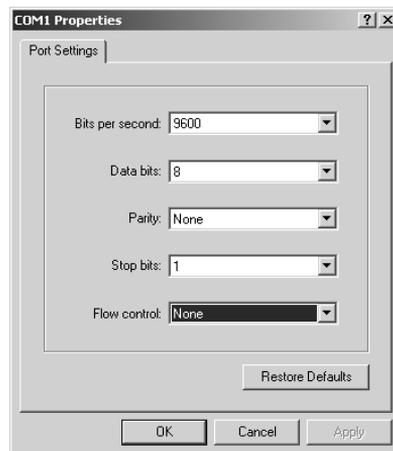
Notice that the bit rate is now set to 9600 and the flow control is set to None. At this point, you can click OK and press the Enter key and you should be connected to your Cisco device console port.
