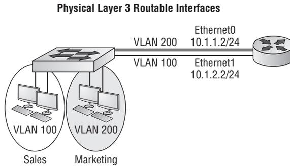
In the figure I used a router to make this work, but I can do this more efficiently by creating a logical layer 3 interface on the switch. These logical interfaces are created for each VLAN and are called switch virtual interfaces, or SVIs. In Figure 7.13, you can see an SVI for VLAN 100 and for VLAN 200.
